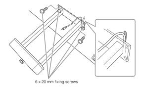
**5** Loosen the four screws that were attached in step 3, and then securely tighten the four screws again while pushing the lyre braces in the direction of arrows as illustrated.
