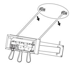
Insert the pedal cord plug into the pedal connector. Insert the plug so the arrow side faces front (toward the keyboard).
