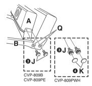
If the screw holes do not align, loosen the other screws and adjust the position of unit B.
