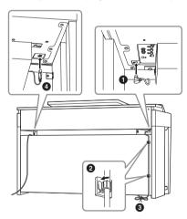
6 Rotate the adjuster until it comes in firm contact with the floor surface.
