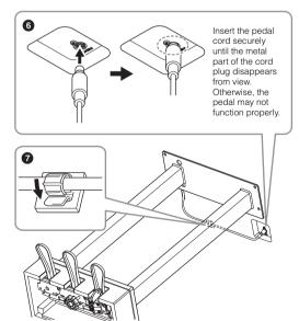
Attach the cord holder to the bottom of the main unit as shown, then clip the holder around the cord.
