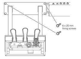
3 Insert the lyre braces into the pedal box recesses and make sure they fit securely.
