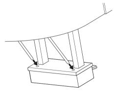
Align the cord with the groove on the unit and attach the backside of the pedal box using the two fixing screws (6 x 20 mm), and then securely tighten the two screws of the front side of the pedal box that were attached in step 5-2.
