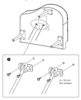
Attach the lyre braces using the four thin screws (4 x 16 mm).
